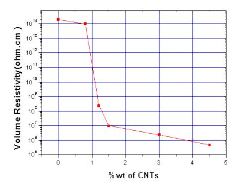
Electrical conductivity of a composite of carbon nanotube masterbatches and high impact polystyrene (HIPS) as a function of the content of carbon nanotubes. The carbon nanotube masterbatches are composed of 10 wt% carbon nanotubes and 90 wt% polystyrene (PS). The composite is prepared by mixing the carbon nanotube masterbatches and HIPS at 210  $^{\circ}$ C with a twin screw extruder. Samples for the resistivity measurement are molded at 210  $^{\circ}$ C and 5 MPa for 10 min.
